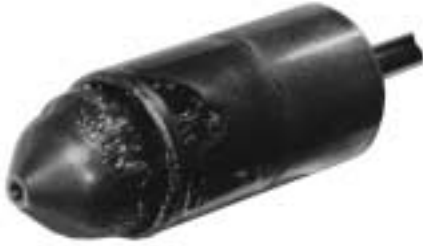
Figure 8. Typical Flashing Damage
