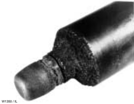
Figure 5. Typical Cavitation Damage
